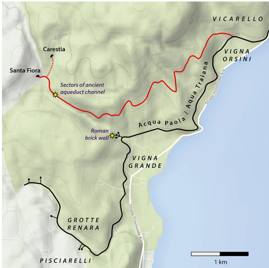
Fig. 11. Northeasterly branch conduit of the Santa Fiora and Carestia sources. Terrain background © 2016 Google.
