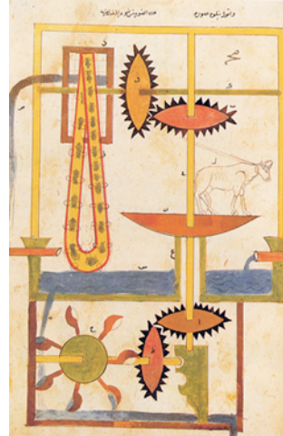
Figure 3a (right). An example of a water-lifting device proposed by Ibn-al-Jazari in “The Book of Knowledge of Ingenious Mechanical Devices”, 1206. Image source: Bodleian Library, MS Greaves 27, folio 101r.
